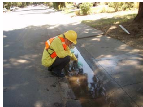
Figure D-4 Collecting grab samples
