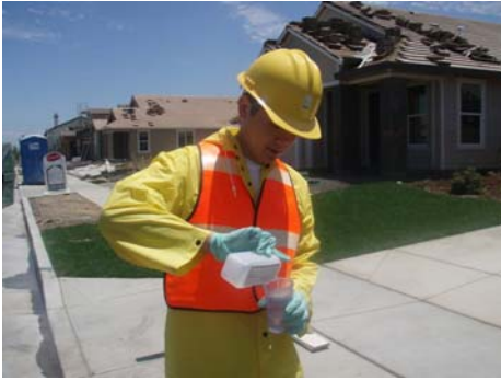
Figure D-5 Transferring sample to field meter sample container
